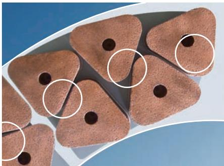
The prism shape of SINTERFLEX disc brake pads guarantees best-possible coverage of the brake disc, regardless of whether wheel-mounted or axle-mounted brake discs are used. The permitted pad overhangs are maintained, even when the bogie is tightly compressed. This prevents particle deposits and wear caused by edge fractures or shearing forces.
