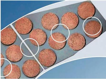
Conventional disc brake pads with cylindrical sinter blocks suffer from edge fractures and cause increased disc and pad wear when using wheel mounted discs. The reason for this is the relatively small coverage of the similarly round and large disc fixing holes.
